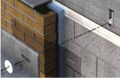
ST-4 Brick relief angle at concrete beam.
