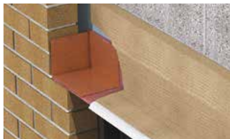
Thru-wall shown with copper end dam
