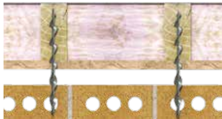
Brick to Wood Stud ( mortar joint or solid brick )
