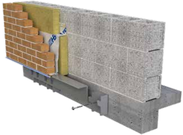
Horizontal Expansion Joint above Slab Edge
